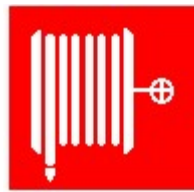
Boca de Incendio Equipada (B.I.E.)
